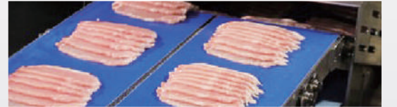
Dual type has individual conveyor control, which allows for fixed weight slicing of materials of different types and shapes at once
