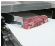
End loss ejection improves yield and work efficiency *End loss ejection refers to the last irregularly shaped portion is ejected without slicing
