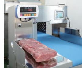
After weighing the ingredients, simply place them on the meat feeding belt and press the start switch
