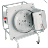
Semi-automatic grinding is possible with dedicated grinding equipment
