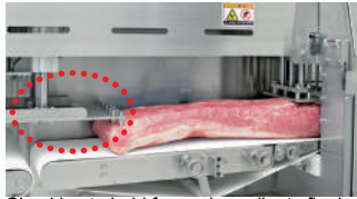
Chucking to hold frozen ingredients firmly
