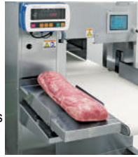
After weighing the ingredients, simply place them on the meat feeding belt and press the start switch
