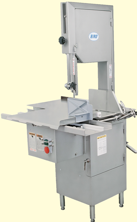
Model 1433 (Movable head structure) Right to left feed.
